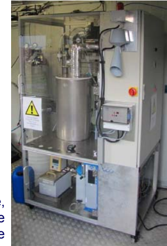
2,5 kW el Biogas- Reformer- System
