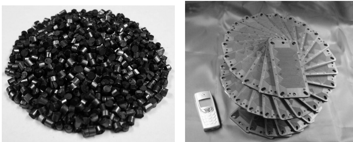
Fig. 3: Granulated compound material and injection moulded bipolar plates
