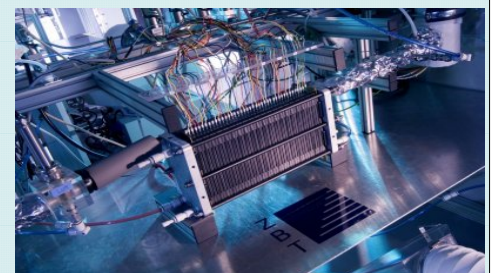
fig.2: typical fuel cell experimental rig at ZBT
