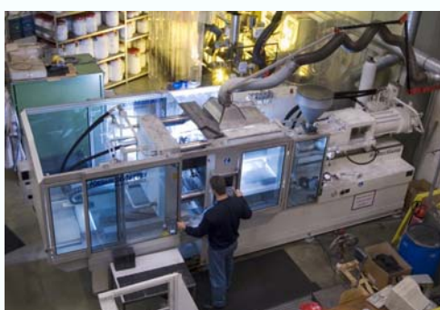
High power injection moulding machine with a clamp force of 300 t and a maximum injection pressure of 3500 bar
