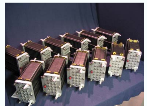
Small series production of fuel cell stacks
