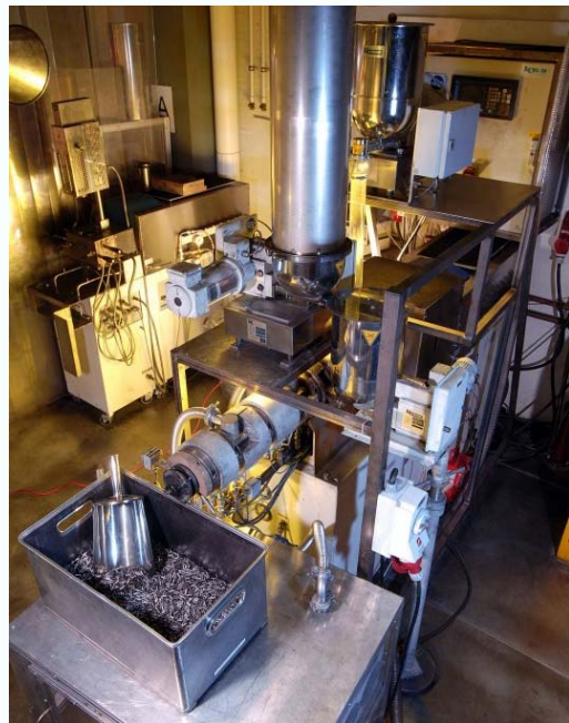
Twin screw extruder with gravimetric metering units, vacuum degassing and self designed nozzle
