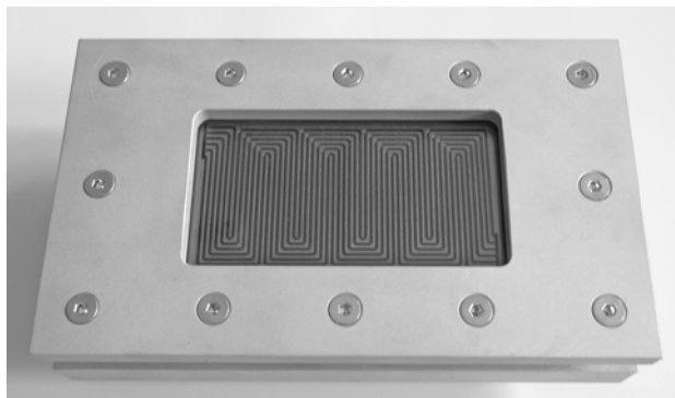
Fig. 1: Photograph of the sealed bipolar plate with optical access to the flow field, with inlet at the bottom right corner and outlet at the top left corner.
