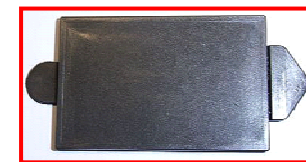
Injection molded samples for three-point bending test
