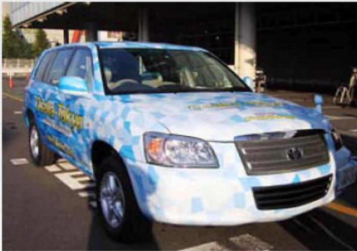
The cruising range has been significantly improved by increasing hydrogen tank pressure (35 MPa => 70 MPa) and system efficiency. (about 300 km => 500 km with practical driving cycle)
