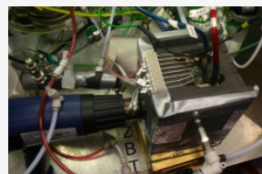
Fig. 9: Test of the 7-cell HT-PEM stack
