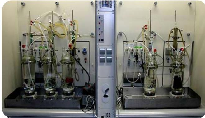
Ex-situ accelerated ageing ( $H_2SO_4$  @80°C or  $H_3PO_4$  c=85% @ 180 °C)
